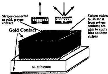
CFH4 Fig. 1 Schematic of the single-element phase-modulator grating device. Insets depict the response of the reflected beam with zero bias and positive bias.
